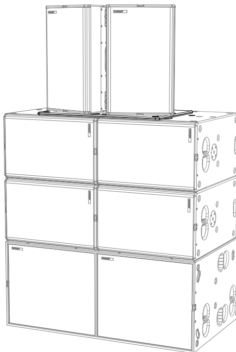
Figure 4.10.1 - System setup BSX loudspeaker with B30 loudspeakers cross
