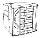
1×6.5" LF | 5×1" HF Drivers 90 - 20000 Hz Frequency range Power capacity program/peak 400/800W Impedance 24 Ω Coverage (h × v) 120° × 10° Sensitivity 1 W/1 m 99 dB SPLmax/1m 129 dB Connection speakON™ NL4 1± Dimensions ( $H \times W \times D$ )  $200 \times 200 \times 260 \,\text{mm} \mid 7.9 \times 7.9 \times 10.2 \,\text{in}$ Weight 5.5 kg | 12 lbs Finish Warnex texture paint (RAL colors optional)
