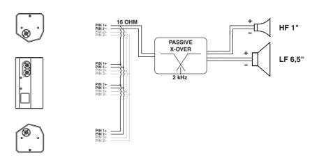
Figure 3.2 - Wiring diagram
