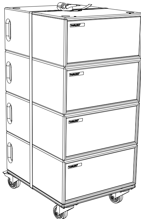
Figure 4.1 - Transport setup B14 loudspeaker with QDB14
