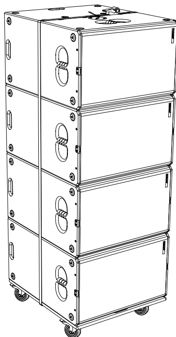
Figure 4.1.1 - Transport setup B30 or VERAS30 loudspeaker with QDB30
