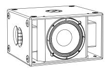
1× 10" LF **Drivers** B10A: 40 - 400 Hz | B10P: 40 - 200 Hz Frequency range Power capacity program/peak 700/1400W B10A:  $8\Omega$  (optional  $2 \times 16\Omega$ ) Impedance B10P:  $1 \times 6\Omega / 2 \times 12\Omega$  switchable Sensitivity 1W/1m 91 dB SPLmax / 1 m 123 dB Connection B10A: speakON® NL4 2± | B10P: speakON® NL4 1± Dimensions (H × W × D) 304 × 504 × 440 mm  $11.97 \times 19.84 \times 17.32$  in Weight B10A: 16,1 kg / 35.49 lbs | B10P: 20,1 kg / 44.31 lbs
