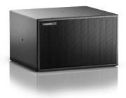
The dimensions of the smallest TW AUDiO installation sub let not assume such a performance. The B10i delivers tight, punsky focused bass from a box barely larger than a microwave oven. Its specifically developed long excursion 10" cone driver with an 3" dual voice coil delivers a usable frequency response down to 40 Hz. This makes the B10i a perfect match for restaurants, clubs and many other applications as main sub or discretely distributed as part of a larger system.
