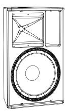
Drivers 1× 15" LF | 1× 1,4" HF with 3" diaphragm 50 - 19000 Hz Frequency range Power capacity program/peak 800/1600W Impedance 8Ω  $75^{\circ} \times 50^{\circ}$  rotatable Coverage  $(h \times v)$ Sensitivity 1W/1m 99 dB SPLmax / 1m 131 dB Connection speakON® NL4 1± Dimensions ( $H \times W \times D$ ) 706 × 440 × 374 mm | 27.8 × 17.32 × 14.72 in Weight 24.9 kg | 54.9 lbs Finish Warnex textured paint (RAL colors optional) Accessories see twaudio.com
