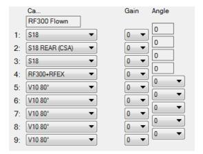
The DSP settings can be changed in the "Filter Settings" Tab. LF DSP preset is set by default to "flat", but can be changed to "cut" or "full" operation mode. If V10P is used, the operation mode and the HF attenuation can be changed in this menu as well.
