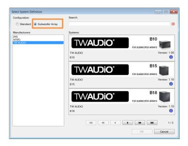
Besides the "Subwoofer Arrays" which contains only single boxes, it is possible to add subwoofers in "Standard" mode as well. This can be done with all subwoofer GLLs. Subwoofer GLLs which can only be used in "Standard" mode are marked with "For CSA Stacks".
